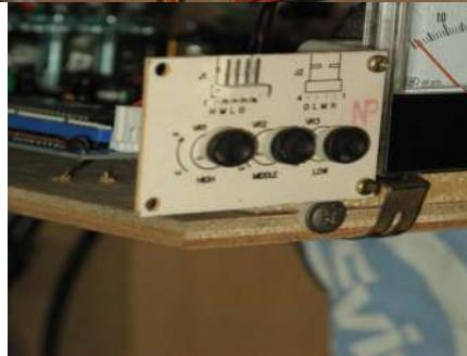
THE VOLTAGE CONTROL BOARD IS EITHER 3 KNOBS ON THE MAIN PCB BOARD OR ON THE SMALL 3 KNOB VOLTAGE ADJUSTMENT BOARD WHICH IS FOUND IN THE COIN MECH AREA.
