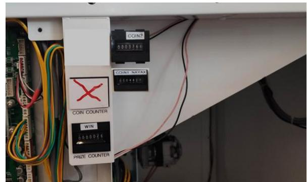
**#8** Test and ensure meters count correctly.
