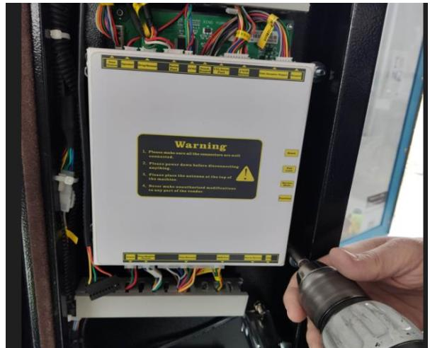
Reinstall the screws on the computer from Step #1 if removed.
