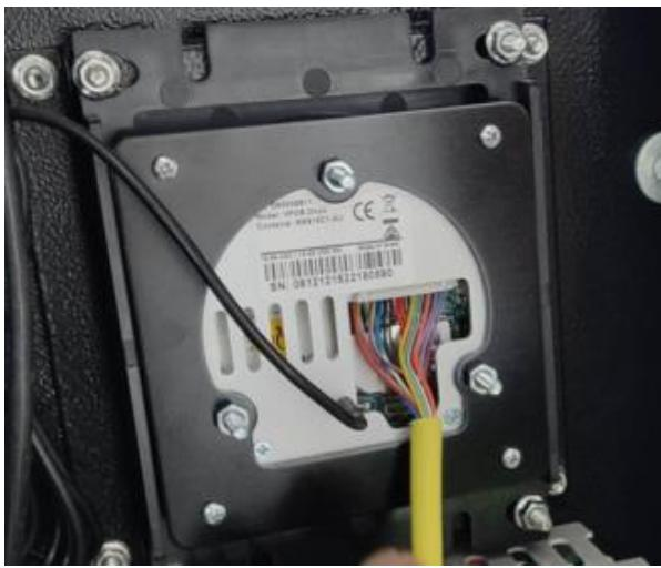
Step # 3 – Disconnect the Coin Mechanism Cable plug.
