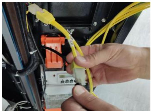
Step # 5 – Connect the plug previously used by the Coin Mechanism to the MALE MDB plug.
