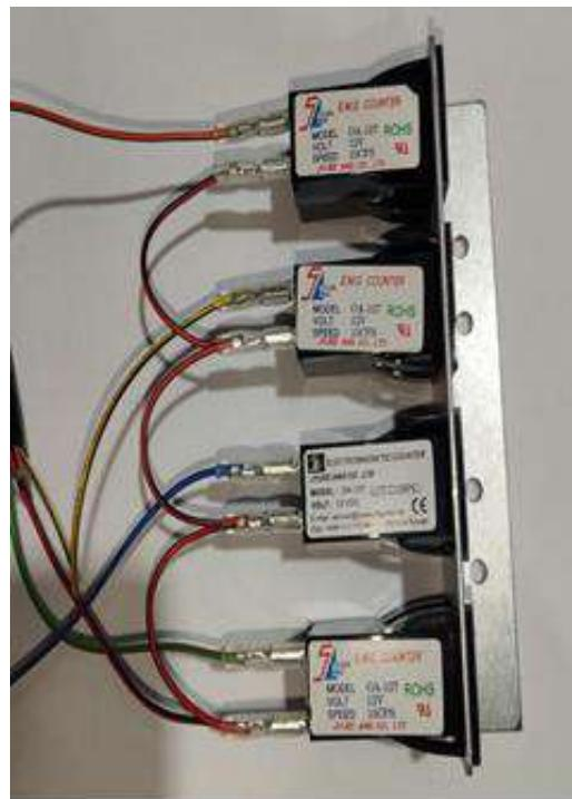
Step #6 – Screw the new Coin Meter holder to the inside wall of the console.
