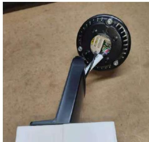
Step #5 – Attach both parts of the holder together.
