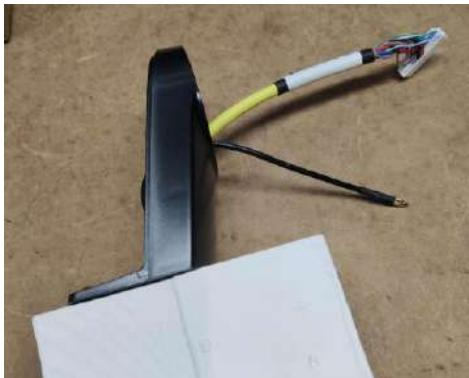
Step #3 – Feed the yellow and black cables through the holder back piece and plug in the cables into the Nayax Reader.
