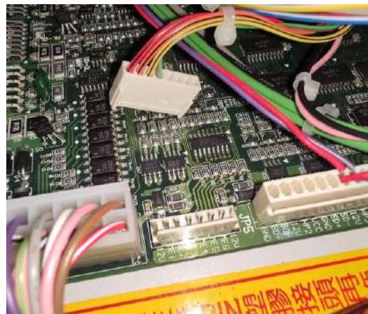
Step #3 – Plug in the new JP5 Loom into the JP5 Socket.
