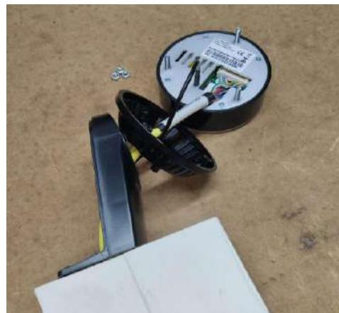
Step #4 – Screw the back holder onto the Nayax Reader.
