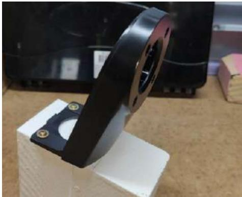
Step #2 – Feed the yellow and black (antenna) cables through the wooden block, and out the front of the holder.
